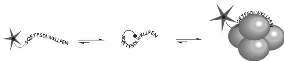
Fig. 9. Principle of operation of PET-biosensors for the specific detection of p53-autoantibodies. Driven by the conformational flexibility the peptide epitope adopts conformations where the fluorophore is efficiently quenched by Trp (W) upon contact formation. The quenched conformation coexists in equilibrium with an open, less quenched conformation. Upon specific binding to the antibody binding site, the peptide adopts a new conformation and charge transfer interactions between tryptophan and the dye are diminished. As the consequence, the fluorescence intensity increases (right side).
