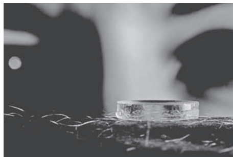
FIGURE 11.1 Microarray patches for transdermal delivery. (Image courtesy of NanoVic, Australia.)
