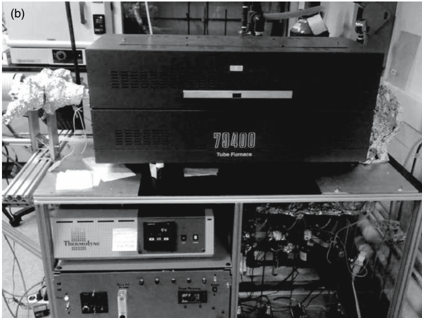
Fig. 4.9 (A) Schematic diagram and (B) photograph of ALD reactor for the deposition of alumina and titania. (courtesy of Prof. C. Summers, School of Materials Science and Engineering, Georgia Institute of Technology)
