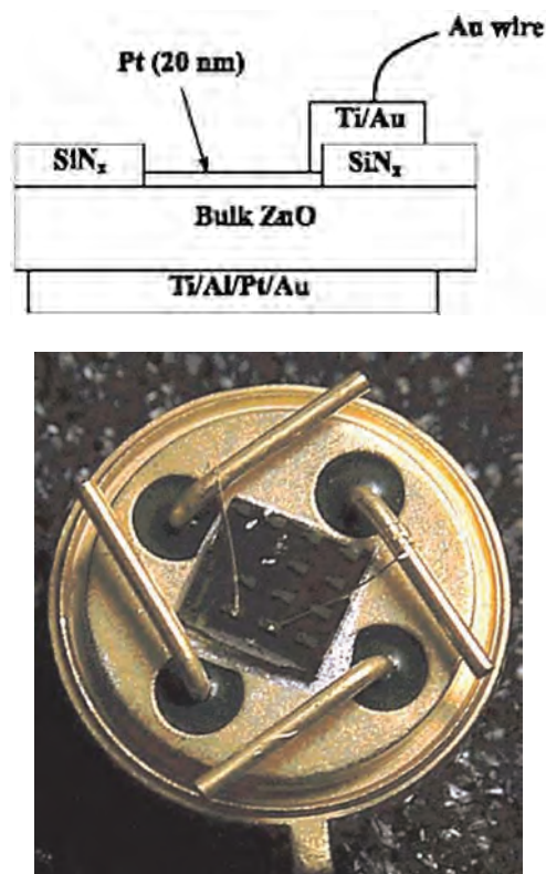
Figure 14.6: Schematic of ZnO Schottky rectifier ( top ) and photograph of packaged device ( bottom ).
