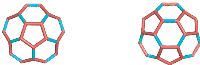
Figure 1-20. From C_{60} fullerene, the two smallest IPR caps can be derived: corannulene- [5:6] 5 (left) and sumanene-[6:(5,6) 3 ] 3 cap (right).
