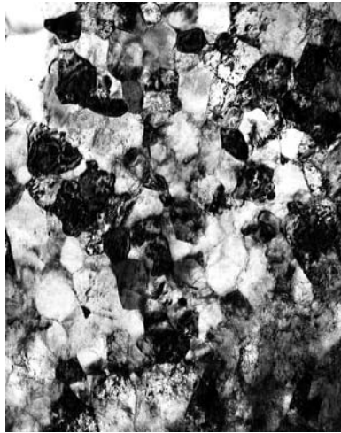
Fig. 1.3 Transmission electron micrograph of nanocrystalline iron produced by consolidation of a nanocrystalline precursor made by ball milling. There is a range of grain sizes, and many of the grains show evidence of the prior plastic work produced by the ball-milling process. The width of the photograph represents 850 nm.
