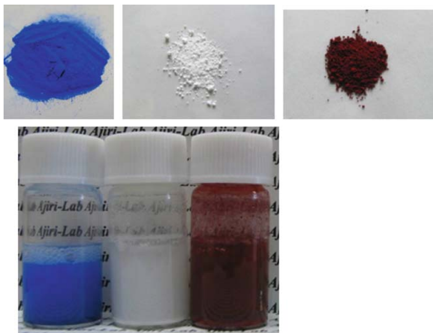
Fig. 11.13. Dispersibility of nanoparticles: \text{CoAl}_2\text{O}_4 (blue); \text{ZnO} (white); \text{Fe}_2\text{O}_3 (brown) in water
