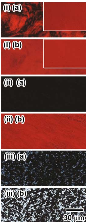
Fig. 2.6. Optical photomicrographs of thermotropic hybrid LC phases of 1/2 hybrids (i) PL1/H2 , (ii) PL1/H5 , and (iii) PL1/H6 at 90°C (a) with a polarizer; (i) – (a) and (b) insets : sheared monodomain
