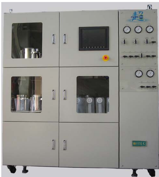
Fig. 11.3. Semipilot plant flow reactor used in the laboratory of T. Adschiri
