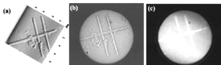
Fig. 6.10. (a) Tapping mode topographic atomic force microscopic image of a magnetic \gamma\text{-Fe}_2\text{O}_3 nanocrystal pattern along with (b) the corresponding mirror electron microscopy (MEM) image collected with electron beam of energy 0.8 eV and (c) X-ray photoemission electron microscopy image obtained by collecting the secondary electrons (energy 0.6 eV) following excitation with 712 eV (Fe L3 edge). The field of view in both cases is 10 \mu\text{m} (reproduced with permission from [942])
