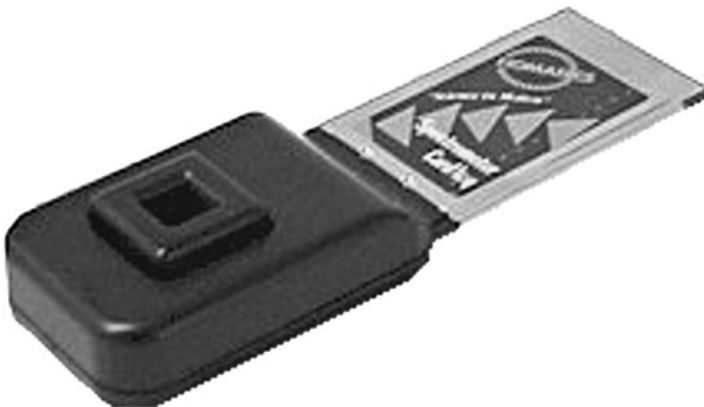
Figure 2.21 MEMS spectrophotometer. (Source: Nomadics, Inc.)
