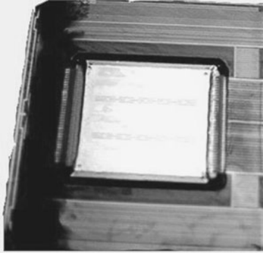
Figure 4.14 Ink-jet chip and connection.
