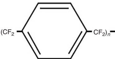
Figure 5.7 Parylene Nova HT structure.
