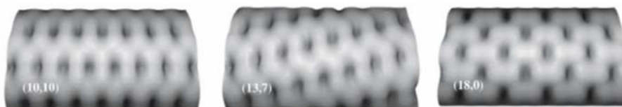
Figure 12. Constant-current (topographic) STM images calculated using a tight-binding Hamiltonian and a point-like tip for an armchair (10,10) , a chiral (13, 7) , and a zig-zag (18, 0) nanotube. (From Ref. [69])
