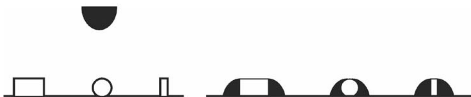
Figure 6. Illustration of the distortion due to tip-sample convolution effects for objects with different shapes. When the object becomes sharper than the tip, the object will generate the image of the tip.
