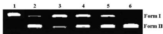
Figure 15.22 Agarose gel electrophoresis of \phi\text{X174} phage DNA ( 20\ \mu\text{M} b.p.) after 8 hours incubation with 100\ \mu\text{M} of zinc complexes (with acetate and chloride anions), without reductant in phosphate buffer, pH 7.2, 37^\circ\text{C} . The oxidative cleavage from form I to form II.
