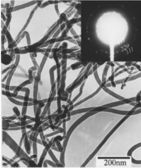
Fig. 10.21. A TEM image of Ge nanowires and a selected-area electron-diffraction pattern (inset) [35].
