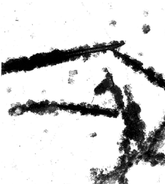
Fig. 6.2. Transmission electron micrograph of the elongated copper nanoparticles coated with CTAPTS.
