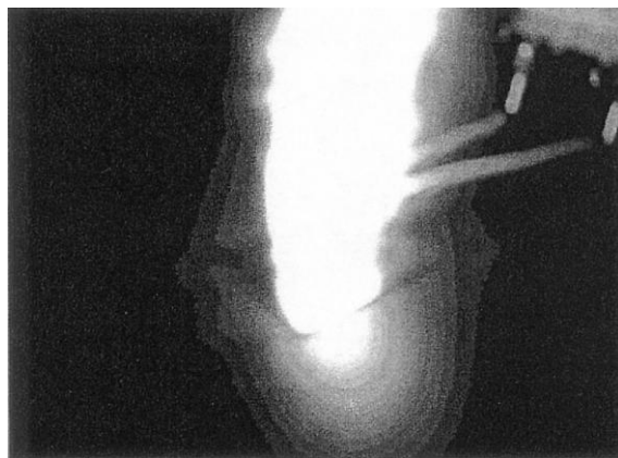
Fig. 16.17. Photograph of the bright flash from explosion of porous silicon treated with \text{Gd}(\text{NO}_3)_3 . Detonation was provided from a transformer (upper right). (M. J. Sailor is thanked for permission to reprint this figure.)
