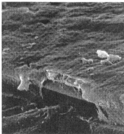
Figure 10. SEM micrograph of a polyethylene/silica/mica hybrid thin film, formed by polymerization of ethylene on a mesoporous silica film-supported titanocene. Reproduced with permission from J. Polym. Sci. Part A: Polym. Chem. 2000 , 38S , 4821. Copyright 2000 Wiley Publishing.
