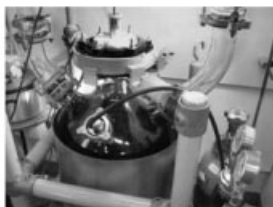
Fig. 2.5 Size-selective formation of airstable Co particles via thermolysis of \text{Co}_2\text{CO}_8 controlled by aluminum alkyl.
