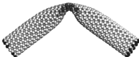
FIGURE 2.9 MD simulation of a large-amplitude transverse deformation of a carbon nanotube, apparently beyond the elastic limit. In fact, the tube snaps back once the computer-generated force is removed, and there is no plastic deformation or permanent damage. (From Yakobson, B. I., Appl. Phys. Lett. 72 , 918–920 (1998), with permission.)
