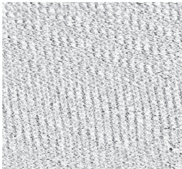
Figure 6. Grayscale STM image of an ordered nanofilm of PTCDA molecules on HOPG surface. The film thickness is 30 Å and the size of the image is 500 \times 500 \text{ Å} . The image was taken in the constant current mode in air with a tip current of 300 pA and a voltage of 150 mV. PTCDA grows in a layer-by-layer fashion on HOPG.
