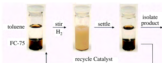
Figure 21. Illustration of the approach used to carry out fluorous biphasic catalysis using dendrimer-encapsulated metal nanoparticles modified on their exterior with perfluoroether “ponytails.” Here, the catalyst is a G4-NH 2 PAMAM dendrimer electrostatically functionalized with a perfluoroether fatty acid. Reprinted with permission from [15], R. M. Crooks et al., Acc. Chem. Res. 34, 181 (2001). © 2001, American Chemical Society.
