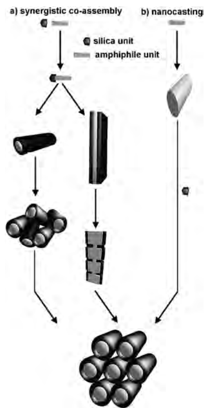
Figure 4. Schematic representation of the mechanisms involved in formation of hexagonally ordered porous materials within the scope of templating strategies. One pathway is characterized by an interaction of amphiphile and network precursor leading to the nanostructured composite phase (synergistic coassembly). In the other case, a template structure is formed at first, and imprinted precisely into a solid mold.
