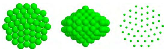
Figure 12. As icosahedra, also decahedra are noncrystalline structures with fivefold symmetries. Decahedra present a single fivefold axis, corresponding to two fivefold vertices. A decahedron is obtained by joining two pentagonal pyramids at their basis. This kind of decahedron has ten triangular close-packed facets, but its shape is far from being spherical. A better structure can be obtained by truncating the sides in such a way that rectangular facets are exposed, and forming reentrances exposing further close-packed facets. In this way a Marks decahedron is obtained. The Marks decahedron of N = 146 atoms is shown: from left to right, top view (along the fivefold axis), side view, and a different representation of the top view, which shows that atoms are perfectly arranged in columns from this perspective. This decahedron has (m, n, p) = (3, 2, 2) : m is the length of the horizontal side of the rectangular facets (see the middle panel) in number of atoms; n is the length of the vertical side of the rectangular facets; p is the depth of the reentrance (see the left panel), with p = 1 corresponding to no reentrance at all.
