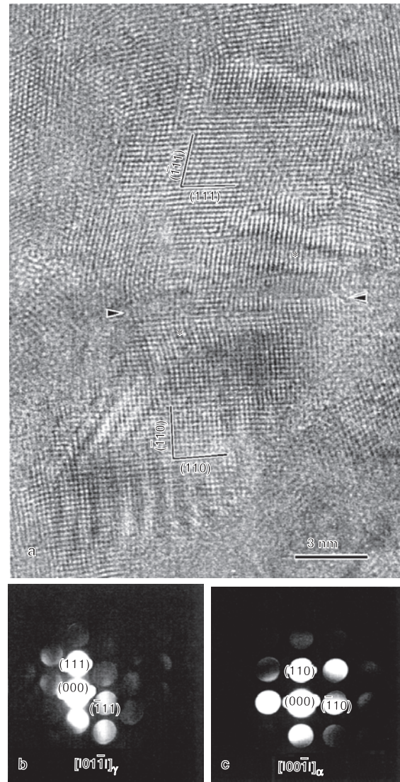
Figure 5. An HRTEM image of an interface between bcc- and fcc-Fe rich Cu in the sample milled for 30 h. (a) The NW orientation relationships, that is, [001]_{\alpha} // [011]_{\gamma} and (110)_{\alpha} // (111)_{\gamma} , exist between the two phases. The arrows indicate the interfaces and asterisks mark lattice distortion regions. The EDPs and EDS from fcc-Fe rich Cu (top) and bcc-Fe rich Cu (bottom) are shown in (b), (d), (c), and (e), respectively [64].
