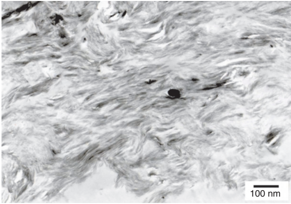
Figure 18. TEM of platelet edge to face association at 5% montmorillonite.
