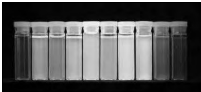
Figure 5. Ten distinguishable emission colors of ZnS-capped CdSe QDs excited with a near-ultraviolet lamp. From left to right (blue to red), the emission maxima are located at 443, 473, 481, 500, 518, 543, 565, 587, 610, and 655 nm. Reprinted with permission from [27], M. Y. Han et al., Nat. Biotechnol. 19, 631 (2001). © 2001, Macmillan Magazines Ltd.
