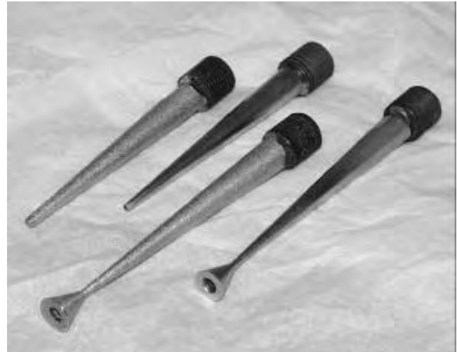
Figure 8. Self-lubricating nanocrystalline nickel + molybdenum disulfide composite coating on hydraulic expansion mandrels.
