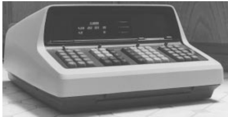
Figure 3-28 HP 9100 series desktop calculator. [Source: http://www.teleport.com/~dgh/91003q.jpg .]
