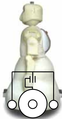
Figure 8. The drive wheels are connected by a jack to the main body and support wheels. The figure shows the inverted pendulum mode.
