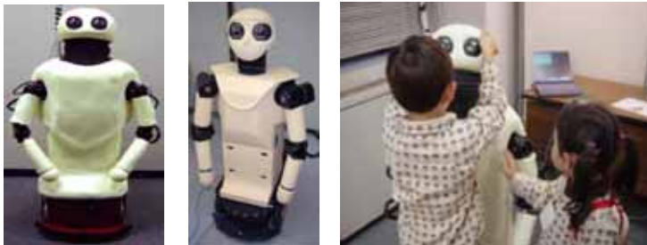
Figure 1. From left to right, Robovie-IIS, Robovie-IIF, and haptic interaction between children and Robovie-IIS.
