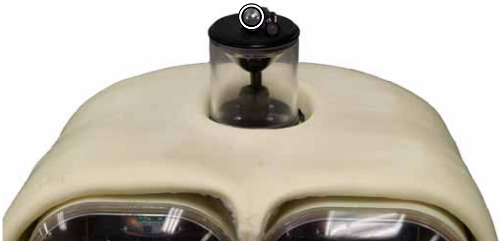
Figure 3. A microphone, attached on a omni-directional mirror, is located on top of the head
