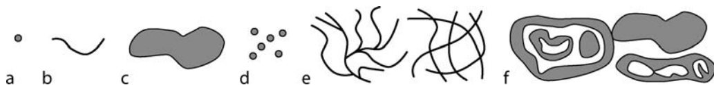
Spatial and Spatio-Temporal Data Models and Languages. Figure 1. Examples of a simple point object (a), a simple line object (b), a simple region object (c), a complex point object (d), a complex line object (e), and a complex region object (f).
