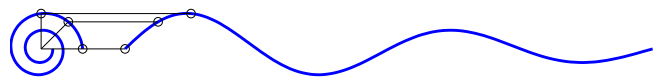
Figure 24.6: A single phasor plotted as a damped two dimensional rotation \mathbf{h}_{t+1} = \gamma \mathbf{R}_\theta \mathbf{h}_t with a damping factor 0 < \gamma < 1 . By taking a projection onto the y axis, the phasor generates a damped sinusoid.
