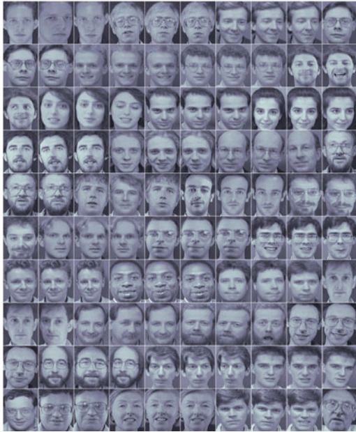
Figure 15.5: 100 of the 120 training images (40 people, with 3 images of each person). Each image consists of 92 \times 112 = 10304 greyscale pixels. The train data is scaled so that, represented as an image, the components of each image sum to 1. The average value of each pixel across all images is 9.70 \times 10^{-5} . This is a subset of the 400 images in the full Olivetti Research Face Database.
