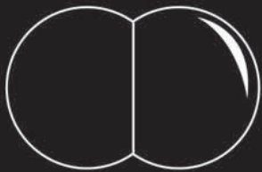
If two bubbles meet in midair, they shrink their surface area by forming a shared, flat wall between them.
