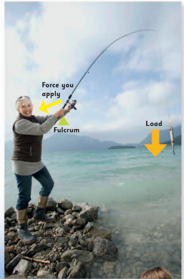
The rod also works as a class 3 lever when you haul in a fish.
