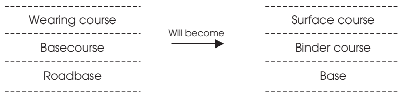
Figure 8.1 Proposed renaming of pavement layers.
