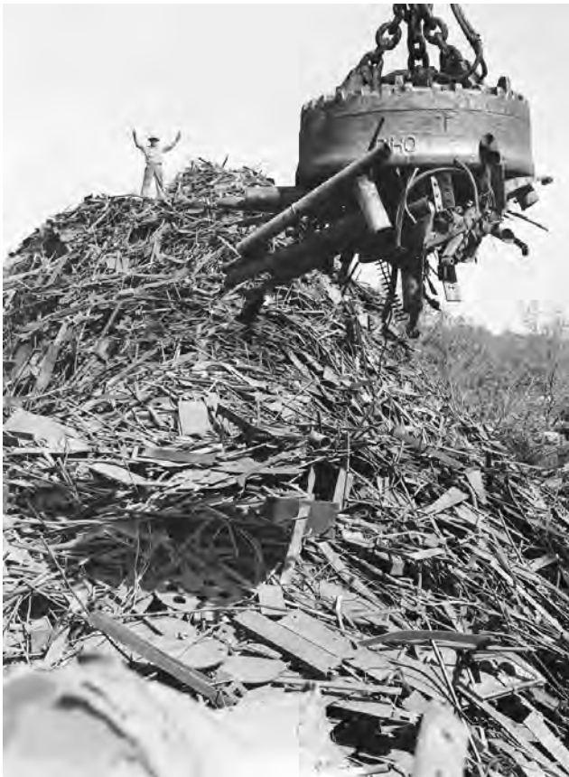
Electricity turns this large piece of metal into a powerful magnet, allowing scrap metal to be easily moved. © Corbis/Bettmann. Reproduced by permission.
