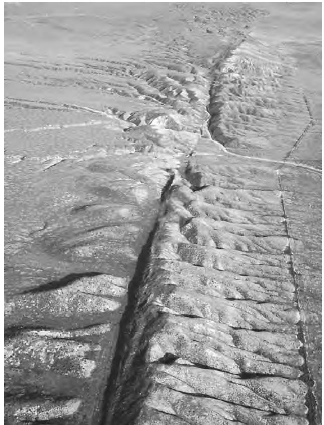
The San Andreas fault is a famous example of a strike-slip fault. Photograph by Robert E. Wallace. U.S. Geological Survey.
