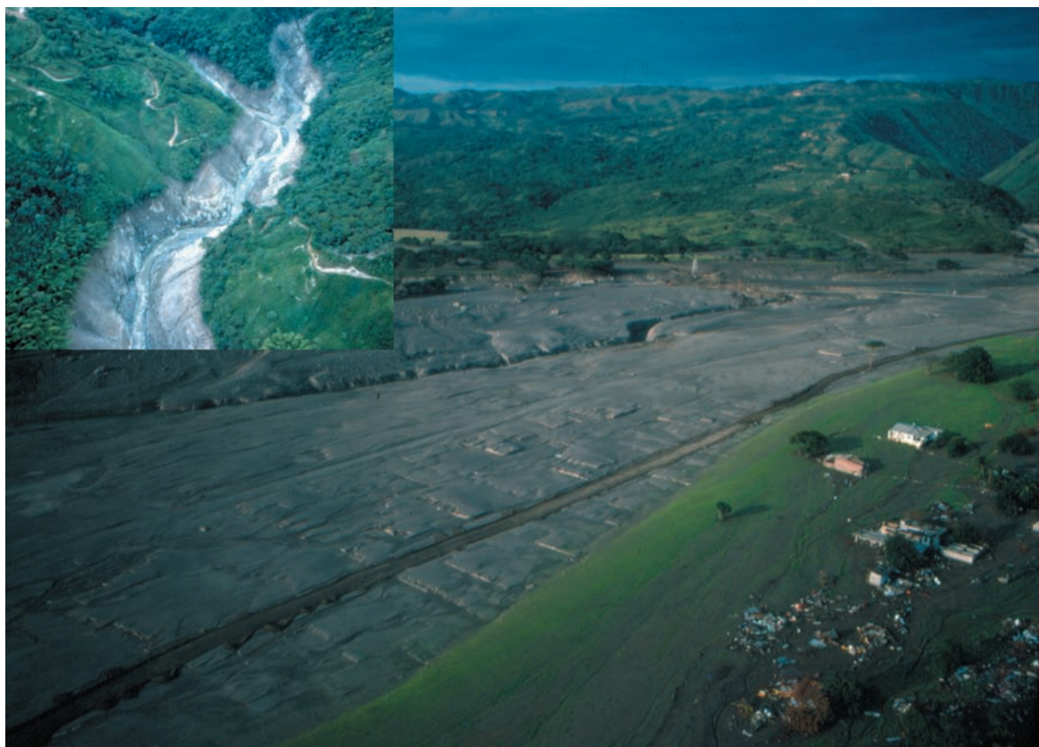
Fig. 11.6 The ruins of Armero, Colombia, after it was destroyed by lahars on the night of November 13, 1985. The lahar from Ruiz volcano was channeled by the Lagunillas River in a narrow flow up to 35 m deep (inset) but was less than 3 m deep where it widened and flowed through the city. The lahar contained entrained boulders more than a meter in diameter, however, which acted like battering rams, destroying three-story-high concrete buildings, of which only the foundations remain. More than 23,000 people perished in Armero that night – but none of the victims would have needed to walk more than 150 m to higher ground and salvation. USGS photos by J. P. Lockwood.
