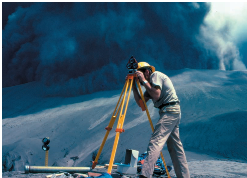
Fig. 1.8 EDM reflector at Pasir Bentang station below the erupting crater of Galunggung, August 1982. A small pyroclastic flow is beginning to cascade down the crater wall, and the thin deposits left by similar small Haws are seen behind the reflector tripod. Note the permanent reflector mounted on stake to left. Photo by Dedy Mulyadi.
