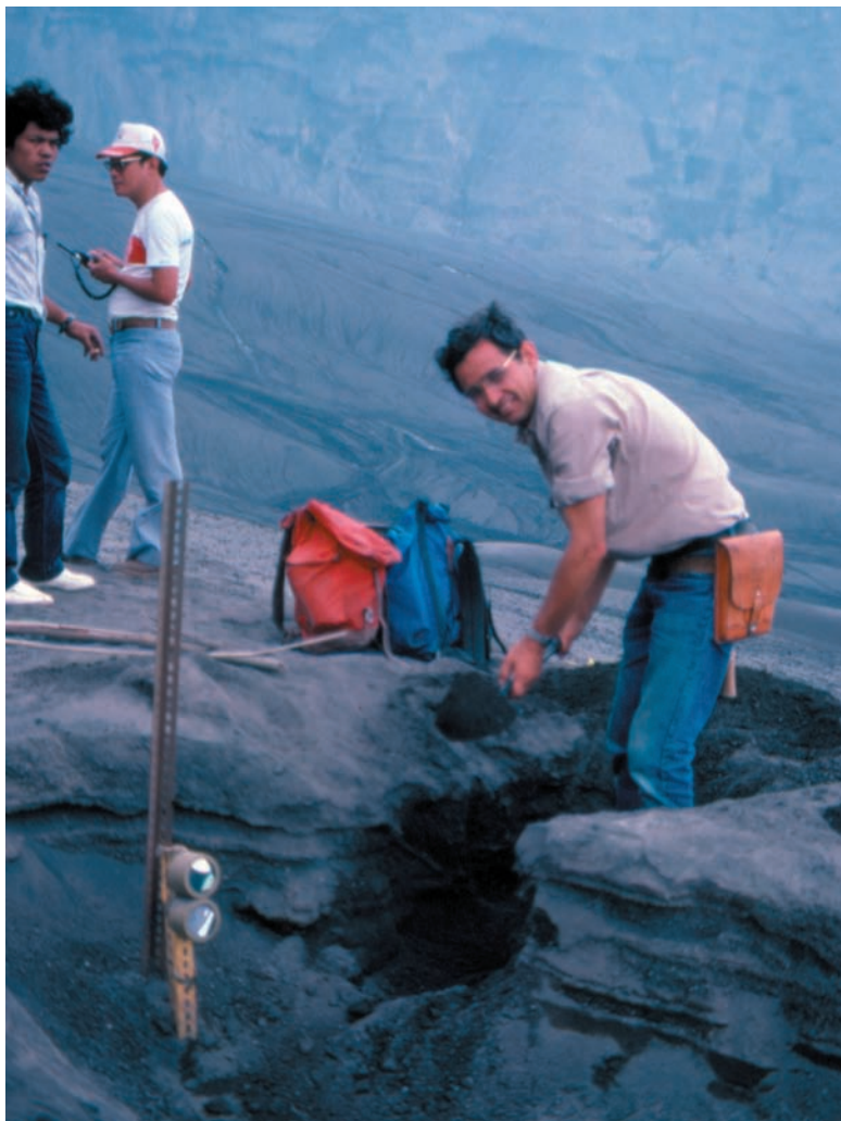
Fig. 1.9 R. I. Tilling excavating line-of-sight path for EDM measurements at Pasir Bentang station, Galunggung, October, 1982. The reflectors had to be re-excavated after every tephra fall event – this is the same reflector that had been above ground two months earlier (Fig. 1.8). USGS photo by J. P. Lockwood.
