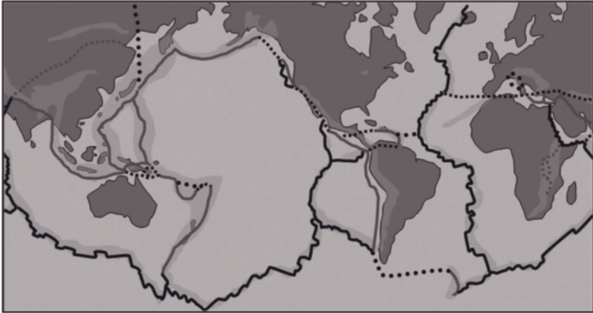
Fig. 8.14 A simplified map of the tectonic plates. The solid black lines represent the locations of spreading ridges, the grey lines are subduction zones, the black square dotted lines are transform boundaries, the grey square dotted lines are collision boundaries, and the large black dots represent uncertain boundaries
