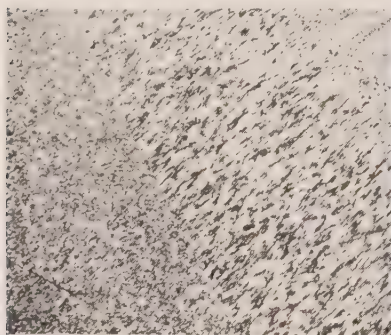
FIG. 96.—Mosaic structure in chalcedony. A "salt and pepper" aggregate of small crystals photographed between crossed nicols.
