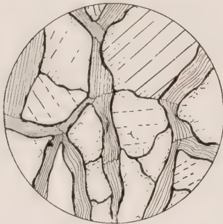
FIG. 119.—Anhedral topaz crystals with broadly spaced cleavage in one direction with penetrating muscovite having closely spaced cleavage in one direction.
