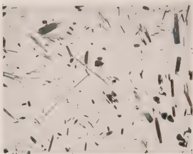
FIG. 222. ( \times 12 ) Tourmaline in quartz.
