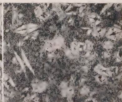
FIG. 111.—Andalusite containing symmetrically arranged carbonaceous inclusions.
