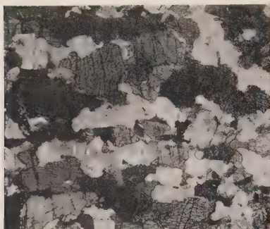
FIG. 106.—Anhedral crystals of hornblende associated with quartz.
