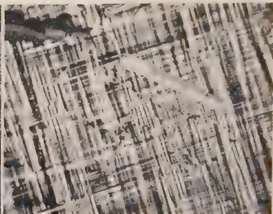
FIG. 169.—( \times 9 ) Microcline section oriented parallel to (001). There are several albite inclusions. ( \times nicols.)
