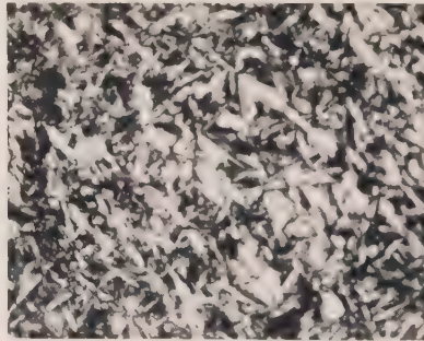
FIG. 251.—( \times 20 ) Antigorite in serpentinite. ( \times nicols.)
