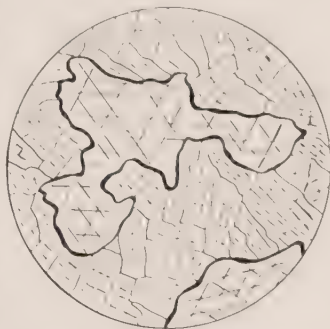
FIG. 123.—Anhydrite (rectangular cleavage) and fluorite (octahedral cleavage) in the same thin section. The octahedral cleavage of fluorite produces a triangular pattern.
