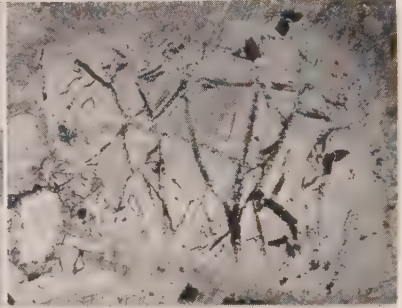
FIG. 139.—(×12) Secondary magnetite in antigorite formed at the expense of olivine.
