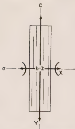
FIG. 258.—Orientation diagram of thomsonite. Section parallel to (010) .
