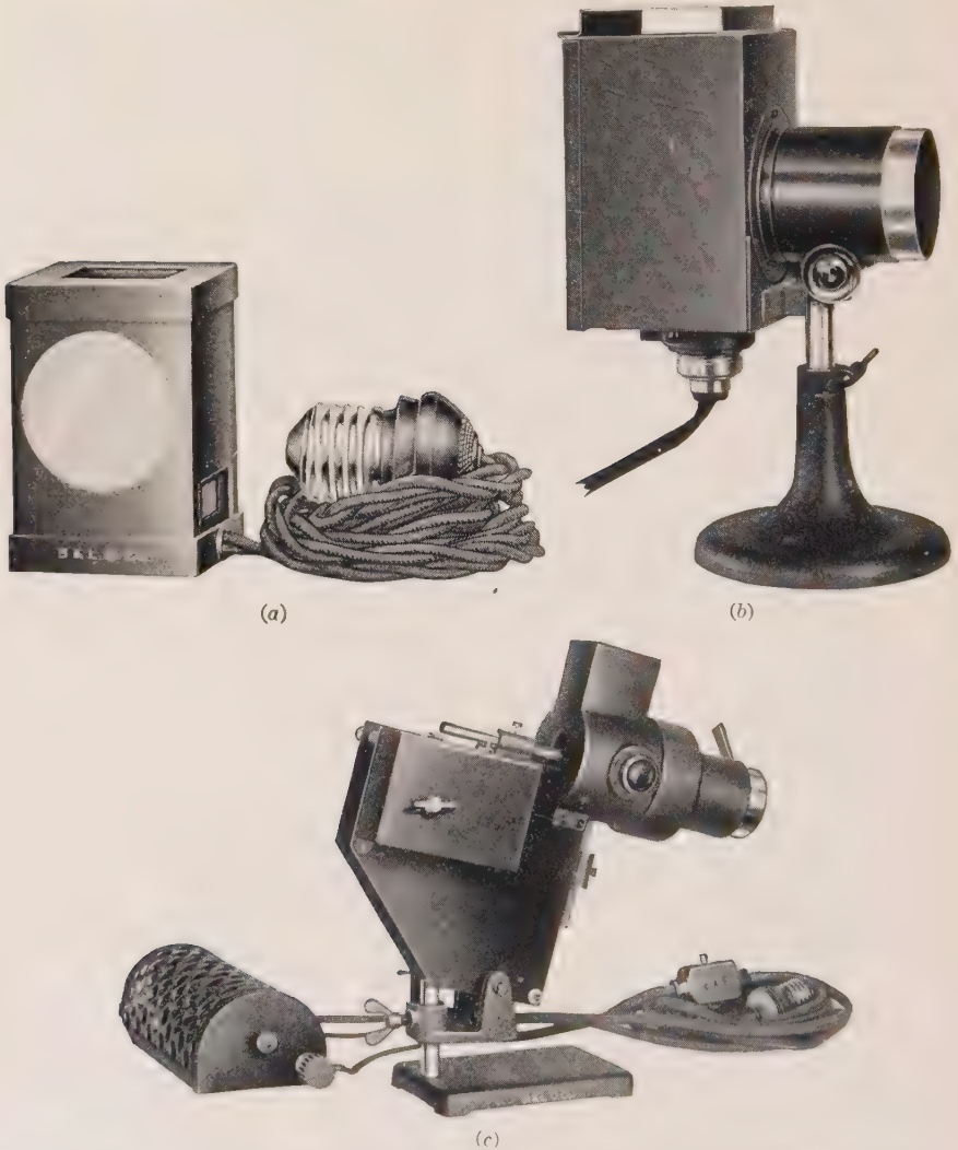
FIG. 25.—Various types of artificial illumination for the microscope. (a) Small substage lamp. (b) Strong lamp for general utility. (c) Arc lamp for special studies or projection. ( Bausch and Lomb Optical Co. )
