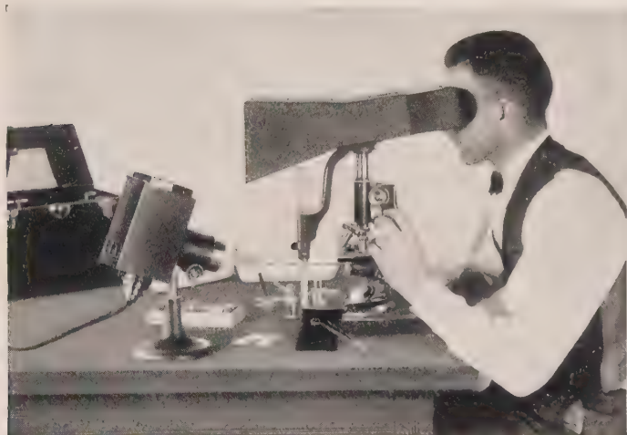
FIG. 22.—The euscope developed originally for biological work but found to be useful for mineralogical work as well. (Bausch and Lomb Optical Co.)
