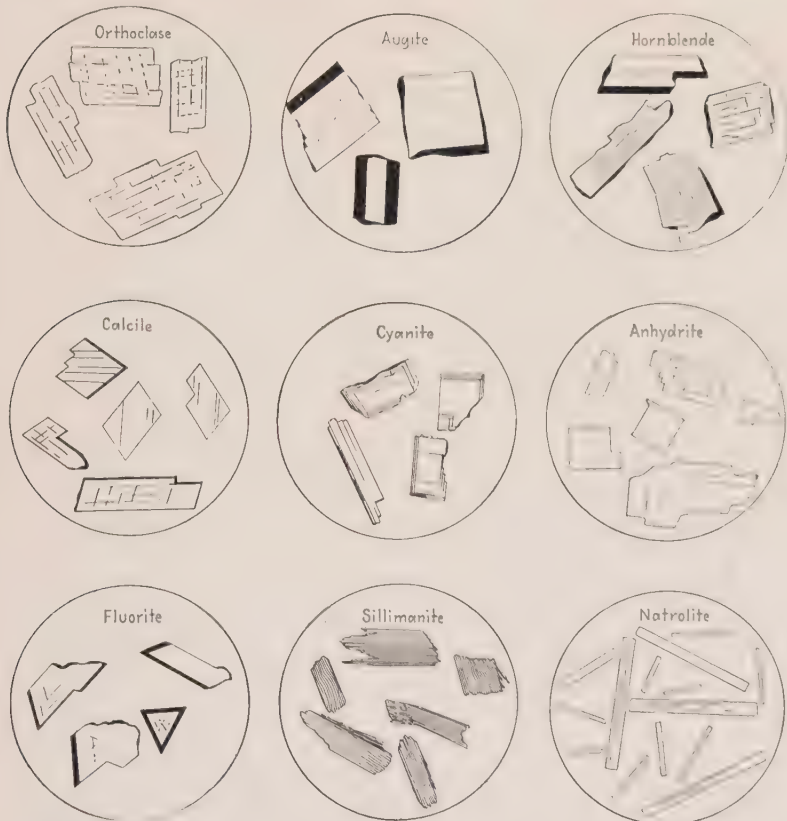
FIG. 118.—Cleavage and fracture fragments. (a) One direction—irregular plates (not illustrated). (b) Two directions—orthoclase, augite, and hornblende. (c) Three directions—kyanite, anhydrite (rectangular), calcite (rhombohedral). (d) Four directions—fluorite (octahedral). (e) Prismatic sillimanite. (f) Acicular—natrolite.
