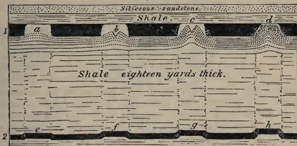
Section of carboniferous strata at Wallsend, Newcastle, showing "creeps." (J. Buddle, Esq.)
