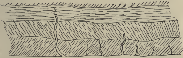
Fissure opening caused by simple contraction.
