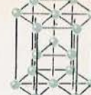
Close-packed Hexagonal (as in zinc)
