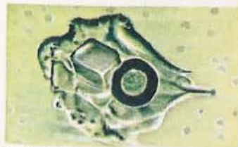
Cubic Salt Crystal and Carbon Dioxide Bubble in Emerald (x195)
