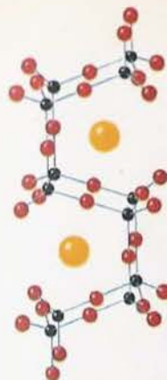
SILICON-OXYGEN FRAMEWORK IN FELDSPARS
