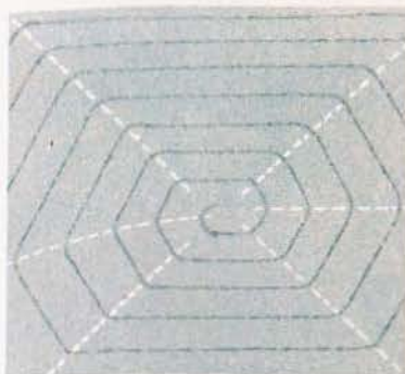
Electron microscope view of screw dislocation on a crystal surface
