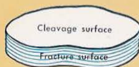
One-directional cleavage as in micas
