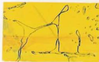
Inclusions in Sphalerite: Rounded areas are gas bubbles. Remainder of inclusions filled with salt water (x14)
