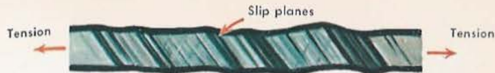
Single crystals can be pulled and stretched because of formation of dislocations (slip planes)
