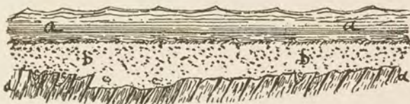
Fig. 6. River Placer. a, a, body of stream; b, b, mud, rocks and coarse material forming bed of stream; c, c, gold-bearing sand and gravel in potholes in d, d, bed rock.
