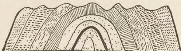
Fig. 7. Fold showing strata running parallel with themselves may be removed by learning to read Nature and being able to discover by the external signs what has taken place in the way of earth disturbances, coupling with this understanding the knowledge of the peculiarity of the rocks of that particular region.
