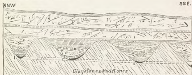
FIG. 38.—SECTION OF THE OLDER DRIFTAL GOLD DEPOSITS NEAR BALLARAT.
