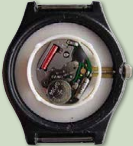
The internal pieces of a quartz wristwatch with the quartz crystal oscillator.
