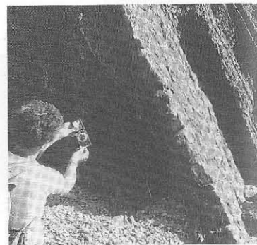
Fig. 2.9b Sighting method. Measurement of the angle of dip of the bedding using the clinometer of the Silva compass aligned parallel to the dip.
