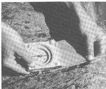
Fig. 2.14 Measurement of the plunge of a minor fold axis by using a pencil to extend the axis.
