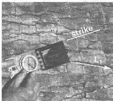
Fig. 2.12b Using the Silva compass as a protractor, place it on the bedding plane and measure the angle between the strike of the bedding and the lineation L_1 on the bedding plane (see text for details).
