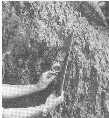
Fig. 2.8b Measurement of the dip of a cleavage plane using a Silva compass and aligning the map board along the cleavage plane.
