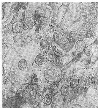
Fig. III.3a Bedding plane in deformed quartzites, showing what were initially circular bedding plane sections of Monocraterion trace fossils, now deformed into strain ellipses with a strain ratio in the bedding plane of 1.3:1.
