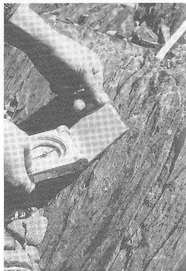
Fig. 2.7 Measure the amount and direction of dip of the bedding by placing the hinged lid of the Freiberg compass flat on the bedding plane.
