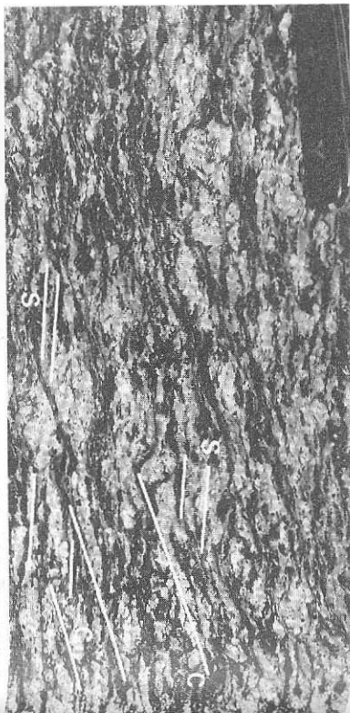
Fig. 6.26b C and S fabrics in a mylonitic granite. A sinistral sense of shear is indicated. C is the shear plane and S is the schistosity plane. (Fig. 6.26a on p. 111)
