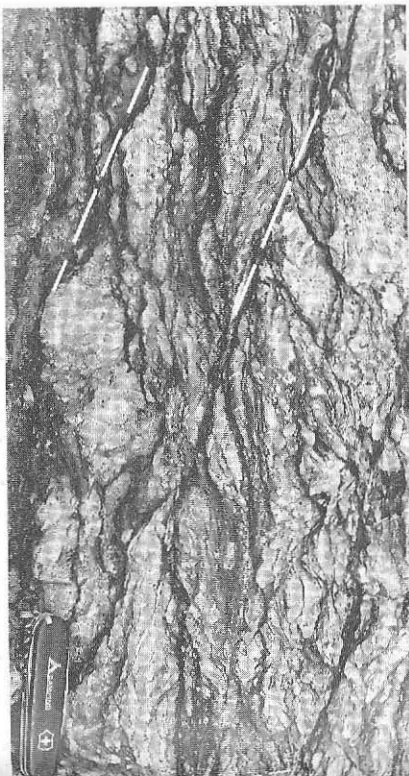
Fig. 6.27b Low-angle shear bands developed in strongly foliated melange (foliation horizontal). (Fig. 6.27a on p. 111)
