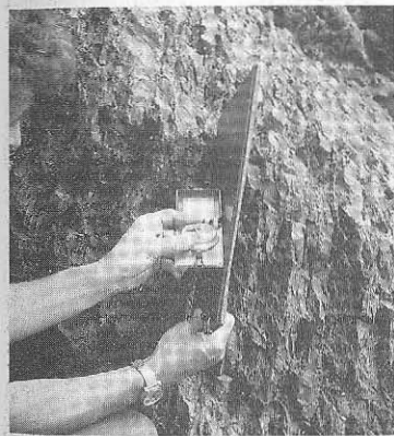
Fig. 2.8a Measurement of the strike of a cleavage plane by aligning the map board along the cleavage plane and measuring the azimuth (direction) of strike using the Silva compass.
