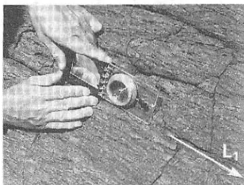
Fig. 2.11c Measure the amount of plunge of the lineation L_1 using the clinometer of the Silva compass.
