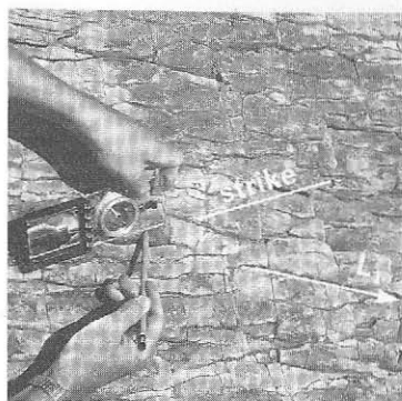
Fig. 2.12a Measurement of the pitch of the bedding/cleavage intersection lineation L_1 on the bedding plane using the Silva compass. Mark the strike line on the bedding plane and determine the strike and dip of the bedding as in Fig. 2.5.
