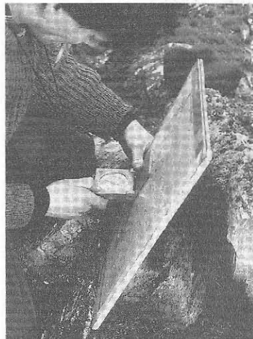
Fig. 2.8c Measurement of the orientation of the axial plane of a minor fold. Align the map board parallel to the fold axial plane and measure the dip direction using the Freiberg compass.
