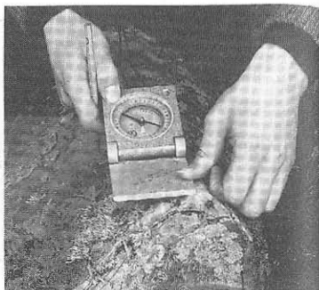
Fig. 2.13 Measurement of the plunge of a minor fold axis by placing the edge of the Freiberg compass on the hinge line.
