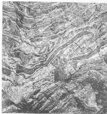
Fig. 3.3c Disharmonic folds of sphalerite layers in galena. There is no continuity along the axial planes between layers. Field of view ca. 1 m.
