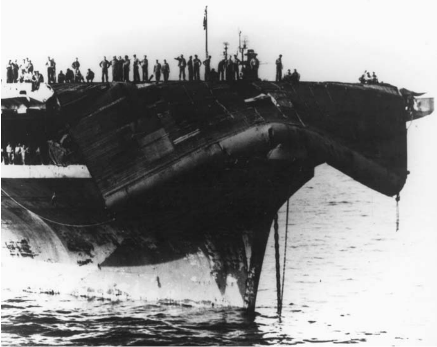
Figure 121 The buckled flight deck of the USS Bennington during a typhoon in the western Pacific in June 1945.
