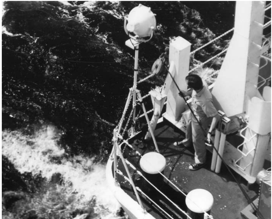
Figure 40 A crew member lowers a magnetometer over the stern of the oceanographic research ship USNS Hayes.
