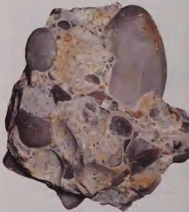
Above: Conglomerates are sedimentary rocks containing large fragments that may be of any rock type.
