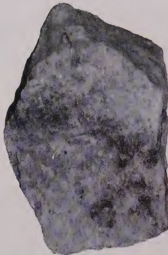
Above: Granulite is composed of light, distinct crystals set in a fine-grained base (matrix).
