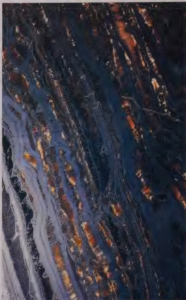
Above: When riebeckite forms in long strands or threads like these it is said to be asbestiform.
