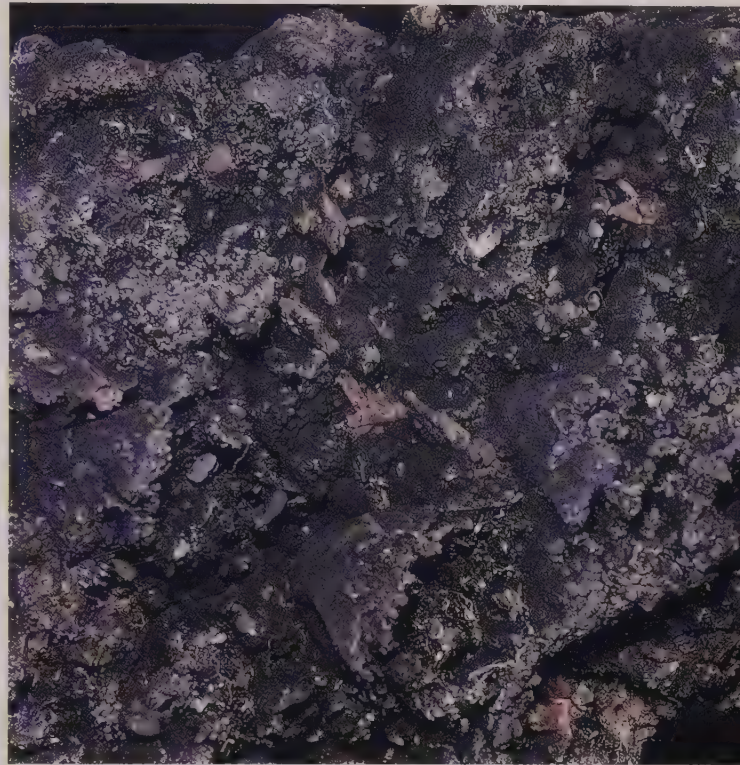
Above: Chalcosite is an opaque, dark gray mineral with a metallic luster.
