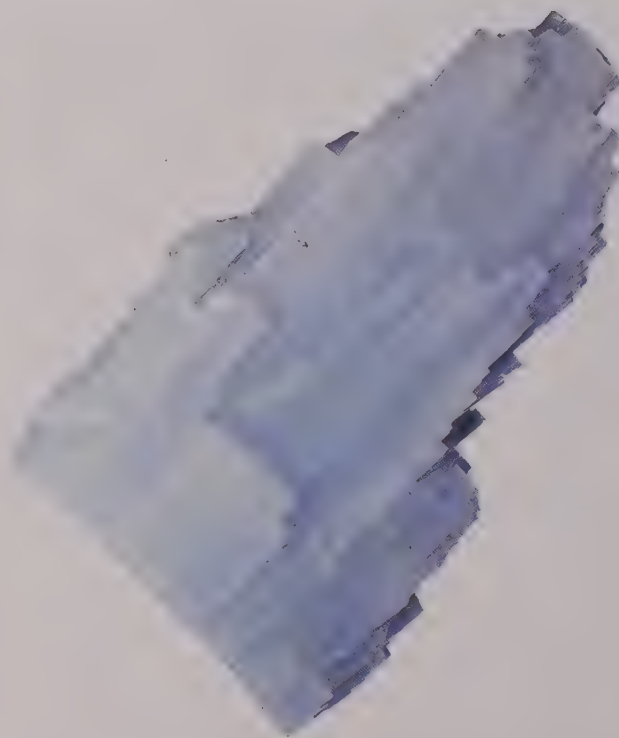
Above: Anhydrite with visible cleavage planes—the lines along which the mineral will break up under pressure.
