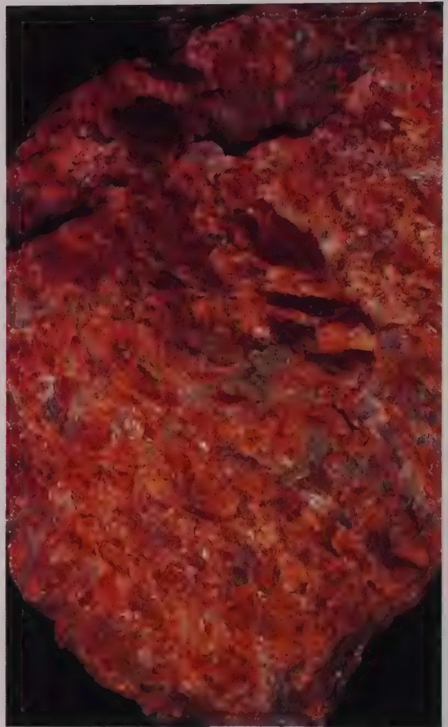
Above: This pegmatite specimen shows very large crystals of feldspar and quartz.
