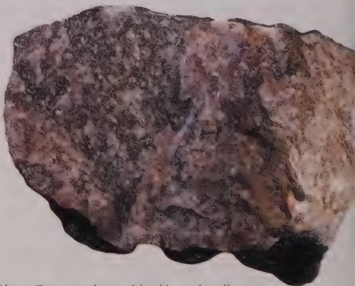
Above: Trona may be grayish white, pale yellow, or pale brown and forms typically in massive, layered habits.
