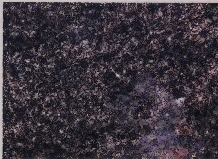
Above: This massive aggregate of pentlandite was extracted from a basic igneous rock formation. Note the metallic luster and the signs of uneven fracture.
