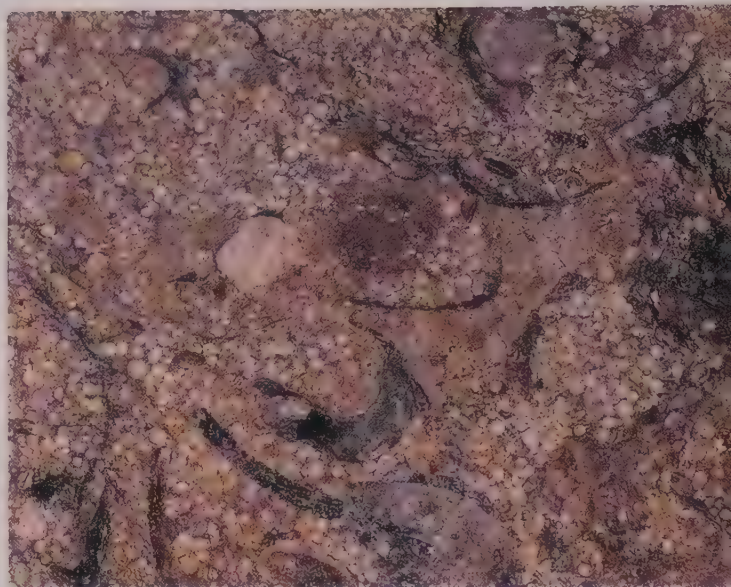
Above: This oolitic limestone from the Jurassic period shows small, rounded ooliths and many shell fragments.
