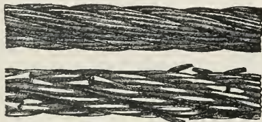
FIGS. 193 and 194.—Wire rope with the ordinary 'lay' before and after use.
