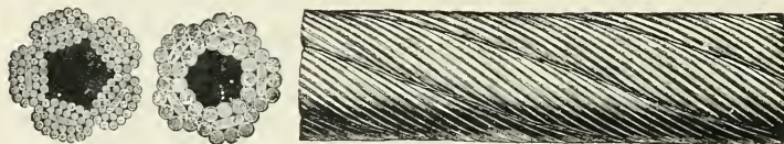
FIGS. 198, 199, 200.—Flattened strand wire rope.
