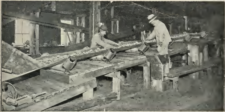
FIG. 172.—Robins Belt Conveyor, used also as a picking table, War Eagle mine, Rossland, B.C.
