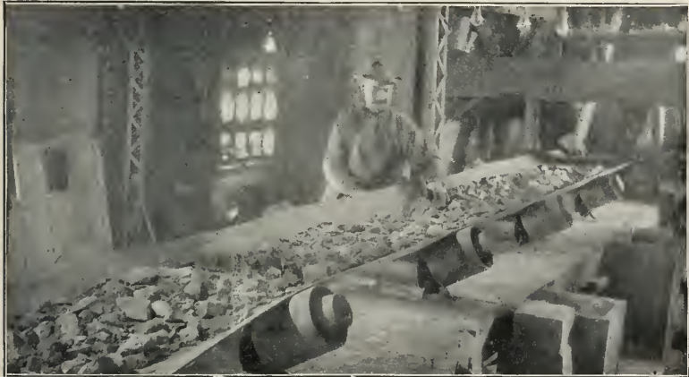
FIG. 173.—Robins Belt Conveyor, used also as a picking table, North Hill iron and zinc mine, Franklin, N.J.
