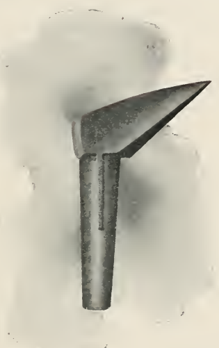
FIG. 95.—Replacable Tooth or Cutter of Hurd's machine.
