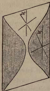
FIG. 46.—AUGITE WITH " HOUR-GLASS STRUCTURE." Section \parallel \infty P \infty . (After L. v. Werveke.)
