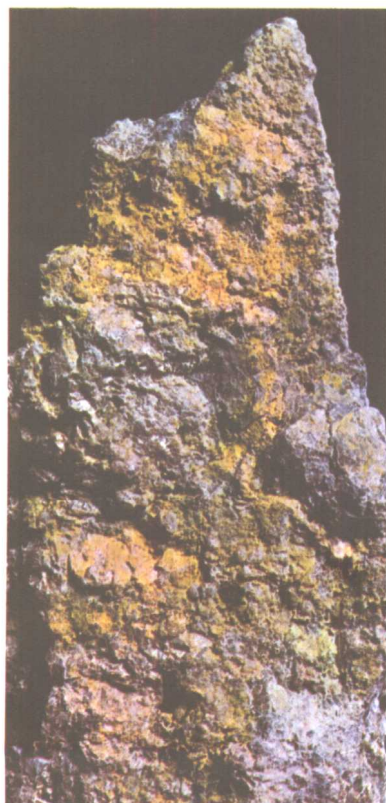
Right: The cadmium sulphide greenockite is usually found as a coating as in this specimen
