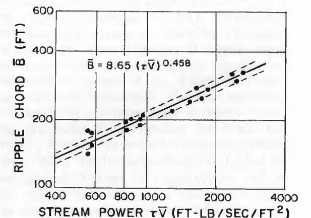
Figure 5.50. Mean ripple chord as a function of stream power. The dashed lines represent one standard error.
