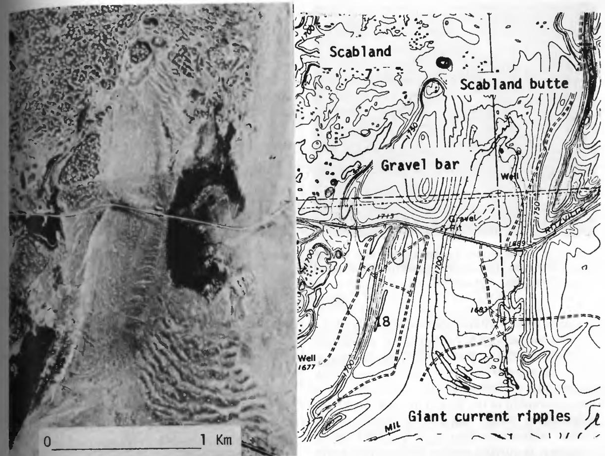
Figure 5.15. Vertical aerial photograph and topographic map of a small pendant bar in the Cheney-Palouse scabland near Macall, Washington. Contour interval is approximately 3 m (10 feet). The bar accumulated downstream from a residual butte of basalt. The bar occurs in sections 7 and 18, T. 18N., R. 38E.
