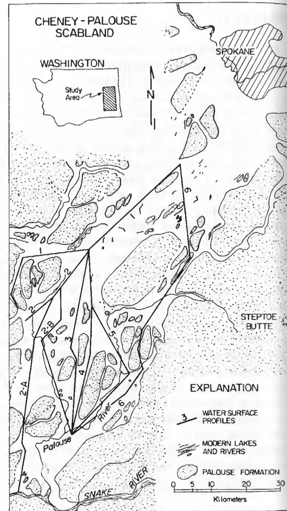
Figure 6.1. Highly generalized sketch map of the Cheney-Palouse scabland tract showing the location of various water-surface profiles that have been determined for the last major Pleistocene flood. Many of the small residual hills of Palouse Formation ("loess islands") have been omitted for simplicity.
