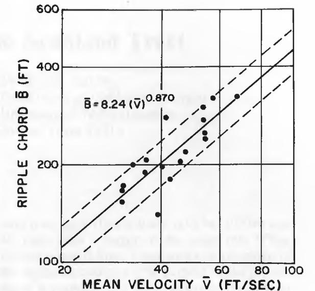
Figure 5.49. Ripple chord as a function of mean flow velocity (discharge velocity) as calculated by the slope-area method. The dashed lines represent one standard error.
