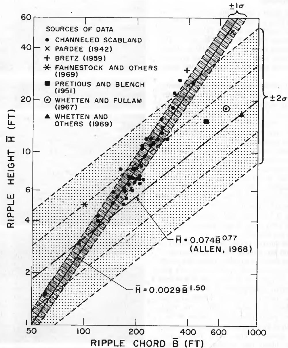
Figure 5.35. Logarithmic relationship of height as a function of chord for 40 sets of giant current ripples. The general relationship for large-scale current ripples determined by Allen (1968) is shown by a dashed line.
