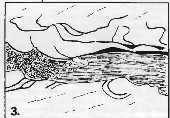
Figure 7.42. Development of experimental scour features in consolidated material through time. 1. Development of linear grooves by longitudinal vortices. 2. Groove enlargement and reduction in number by non-uniform shear stress at the bed. 3. Coalescence of grooves into single channel. Each frame measures about 30 x 40 cm. Redrawn from Shepherd and Schumm (1974, their Fig. 4).
