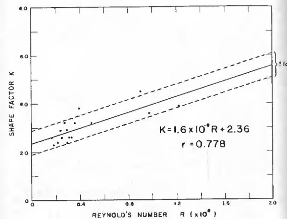
Figure 5.14. Streamlined shape factor  $K$  versus the Reynolds number for maximum scabland flood flows associated with scabland streamlined forms. The dashed lines indicate one standard error.
