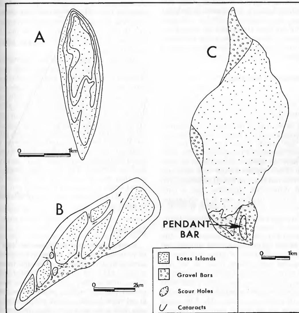
Figure 6.5. Loess island forms in the Cheney-Palouse scabland tract illustrating the three major morphologic types. A. Subfluentially eroded loess island located in the Karakul Hills (Secs. 2, 11, and 14; T. 19N., R. 36E.). B. Partially submerged loess island near Amber Lake
