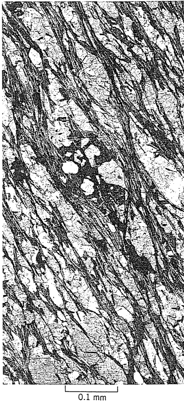
Figure 8.20 Domainal microfabric in schist from Ducktown, Tennessee. Micas form films that envelope aggregates composed principally of quartz. (Photograph by W. C. Laurijssen. From An Outline of Structural Geology by B. E. Hobbs, W. D. Means, and P. F. Williams. Published with permission of John Wiley & Sons, Inc., New York, copyright © 1976.)
