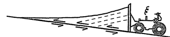
Figure 6.109 The mechanics of development of a thrust belt is analogous to the movement of a mass of snow, sand, or dirt as it piles up and eventually slides en masse in front of the blade of a tractor. This is a far different image than pushing a large rectangular block of rock in front of the blade. [From F. A. Dahlen, J. Suppe, and D. M. Davis, Journal of Geophysical Research , v. 89, figure 3, p. 10,088, copyright © 1984 by American Geophysical Union.]
