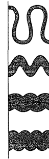
Figure 7.70 The shapes of buckle folds reflect the competency (stiffness) contrast between the stiffer layer and the less competent medium that it occupies. High contrast leads to ptygmatic folds. Low contrast leads to cuscate-lobate folds. Medium contrast creates fold forms that are intermediate between ptygmatic and cuscate-lobate. [Reprinted from The techniques of modern structural geology , v. 2, folds and fractures , J. G. Ramsay and M. I. Huber (1987), Figure 19.14. Copyright © by Harcourt Brace and Company Limited, with permission.]
