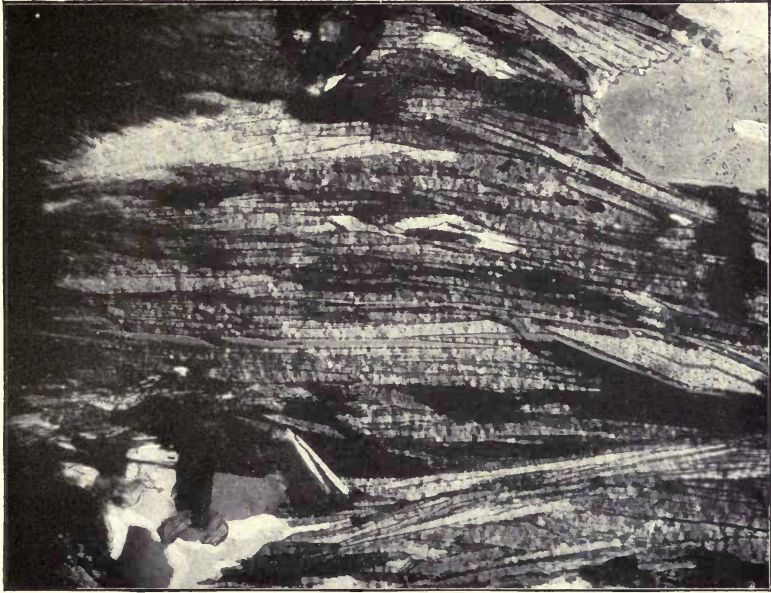
FIG. 39. Photomicrograph of micaceous schist from Hoosac tunnel. The micas, which are entirely new developments by recrystallization, lie in flat plates with their greater diameters roughly parallel. Each individual exhibits several twinning lamellæ. It will be noted that, while there is apparently a bending and irregularity in the mica plates, the individuals are for the most part not deformed, and the impression of irregularity is caused by the individuals feathering out against one another at low angles. This sort of arrangement is frequently seen about rigid particles which have acted as units during deformation, indicating that the arrangement is due to differing stress conditions at different places.
