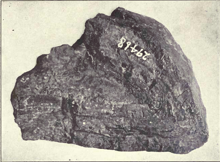
FIG. 53. Folding of brittle and soft layers contrasted in jasper. Note the tension cracks in the brittle layers.
