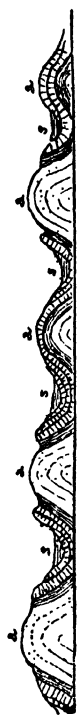
FIG. 148.—VERTICAL FOLDS OF THE JURA MOUNTAINS. a, a, anticlines; s, s, synclines.
