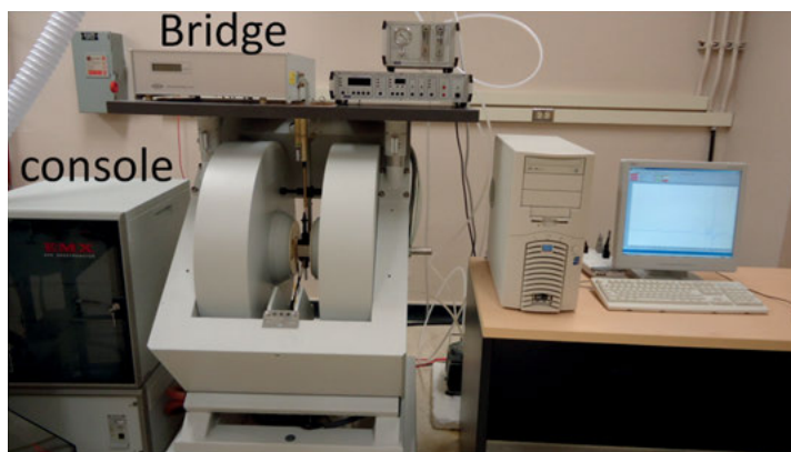
Figure 6. Photograph illustrating the principal components of a CW-EPR spectrometer (Bruker EMX), including the radiation source and the detector in the microwave bridge, the resonance cavity between the magnets, a console containing signal processing and control electronics, and a computer.
