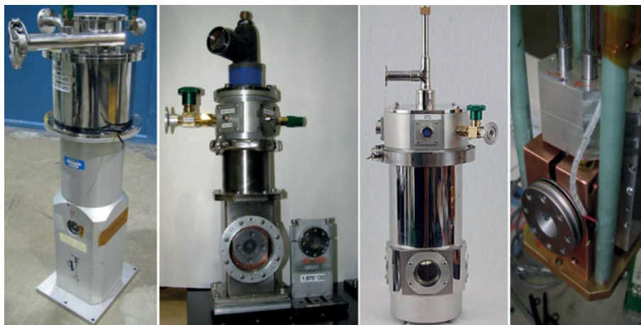
Figure 15. Examples of cryostats at sector 16 (HPCAT) at APS.
