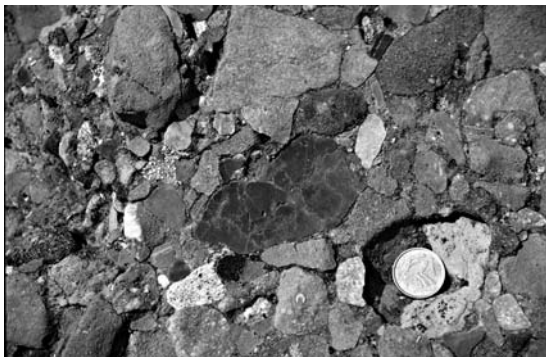
Fig. 2.6 A clast-supported conglomerate: the pebbles are all in contact with each other.
