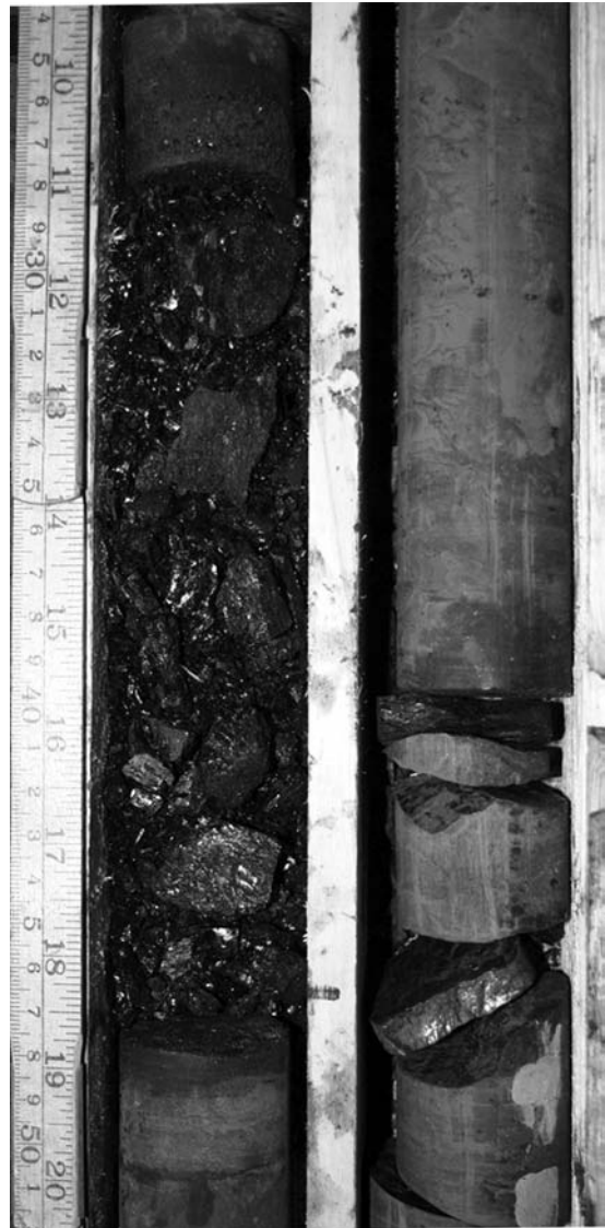
Fig. 22.4 Cores cut by a drill bit and brought to the surface provide information about subsurface strata.
