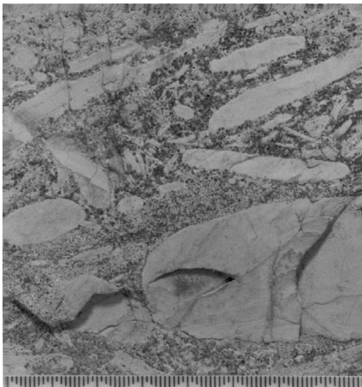
Figure 3.5 Intraclasts (or flakes) of lime mudstone, some tabular, some rounded, in a matrix with quartz grains. Intraformational conglomerate (also called flakestone). Millimetre scale. Late Precambrian, Arctic Norway.
