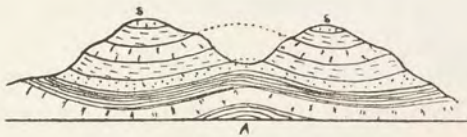
Hills eroded out of folded strata. A , Anti-cline; SS , Syn-clines.
