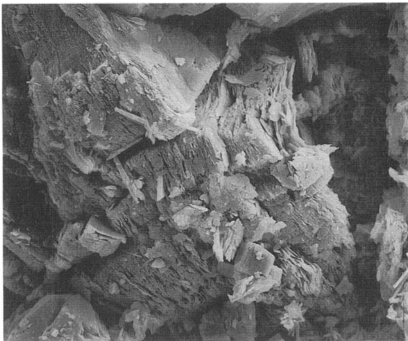
Fig. 5. SEM micrograph of kaolinite observed in the Rannoch Formation. The kaolinite is texturally similar to the detrital kaolinite in Fig. 38 in Keller (1978). Width of photograph = 128 \mu\text{m} .
