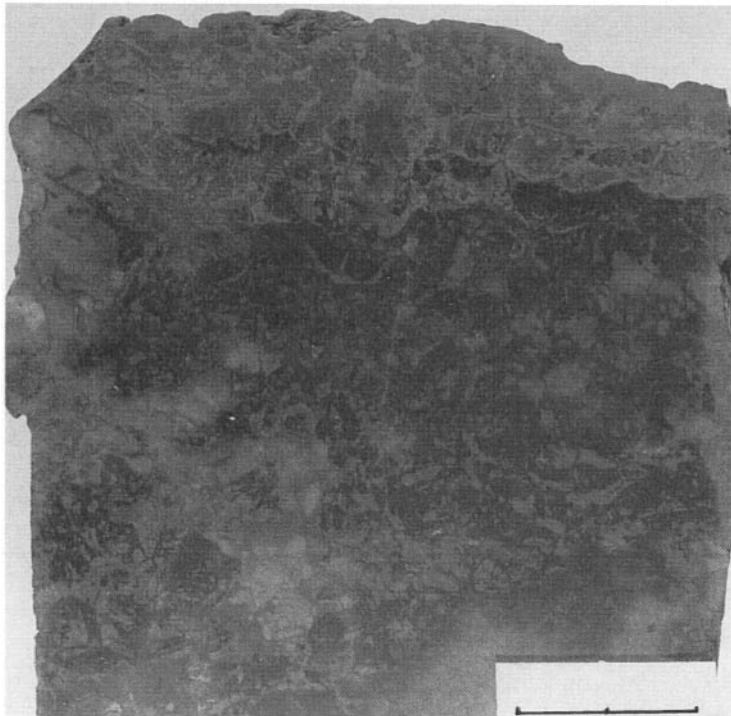
Fig. 5. A polished slab of cementstone bed 13 showing the brecciated macro-fabric. Light clasts are composed of dolomicrite and formed the cementstone body prior to brecciation. Dark areas are reddened matrix composed of silt-sized dolomite crystals. Note the pseudo-lamination in the top 2 cm of the slab which is caused by re-cementation of the breccia fragments. The overall features of this bed are consistent with formation by soil-zone processes (see text). Scale bar = 2 cm.
