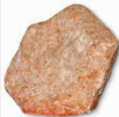
Red dolomite A specimen of dolomite colored with iron oxides and hydroxides
